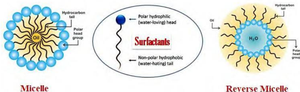
Fig. 1 : Cartoon presentation of surfactant, micelle and reverse micelle.
